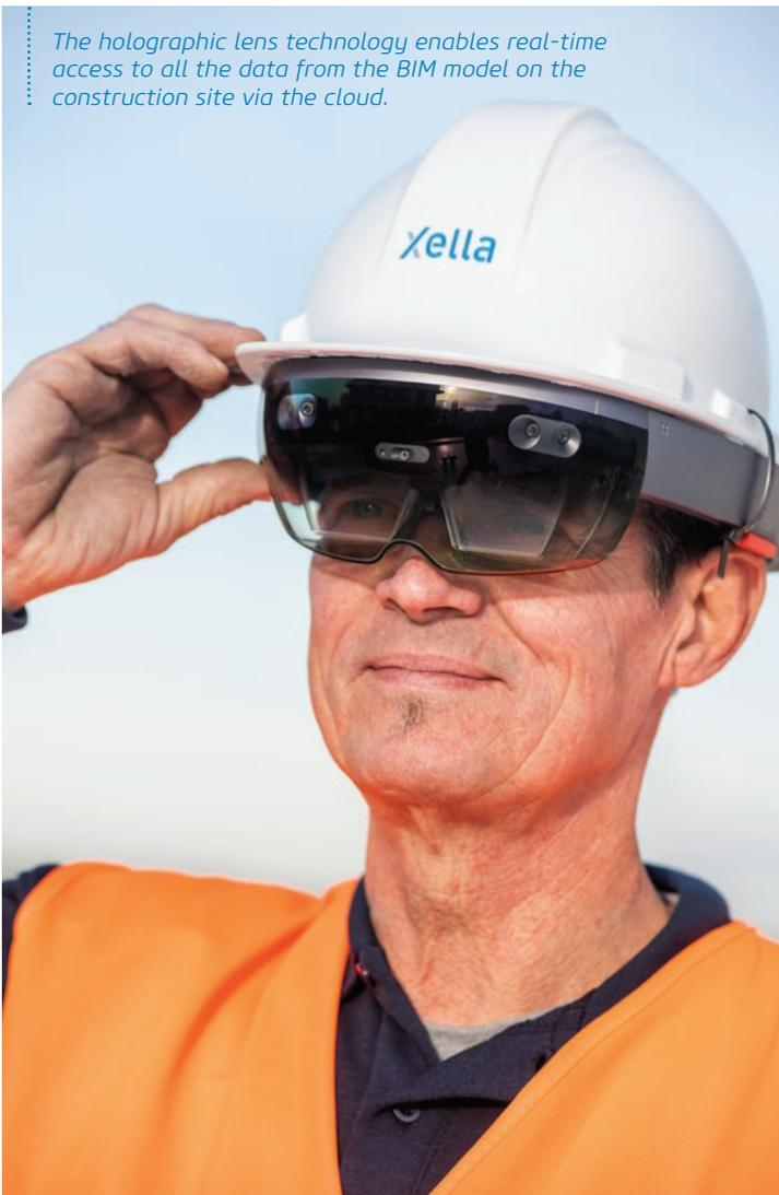
Holographic lens technology enables real-time access to all the data from the BIM model on the construction site via the cloud. For that, construction workers are equipped with a helmet and built-in holographic lens. He can see a holographic representation of the wall or partition to be built. The existing, real environment is also visible to them. This type of Mixed Reality (MR) allows the construction workers to see exactly where and how the wall or partition needs to be erected.
